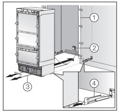
To protect the corners of the installation space, attach the supplied edge protector ① on both sides with adhesive tape. Plug the appliance into the power outlet (2).
